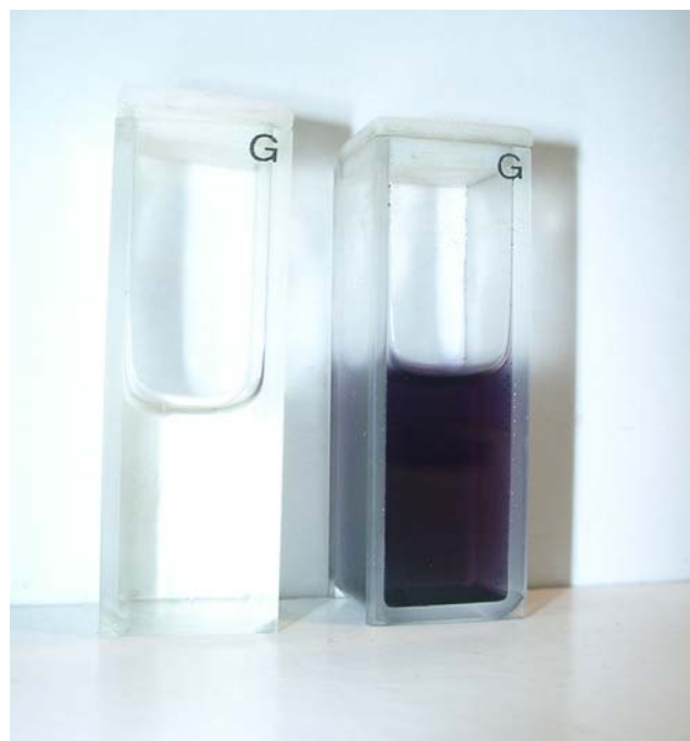
Fig. 3 Polymerization cells containing 1 mM BEDOT-NMCz, 0.1 M LiCF 3 SO 3 acetonitrile solutions after polymerization at 0.75 V (left) and after polymerization at 2 V vs Ag wire (right)
